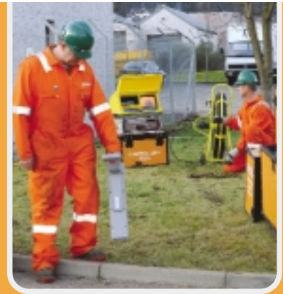
A locator can be used by the operator to track the camera unit to a depth of 5 metres
